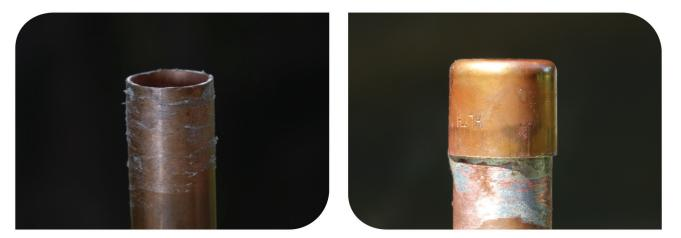
• Using one of 4.5" piece of pipe attempt to solder without cleaning the copper. Note the quality of solder joint
