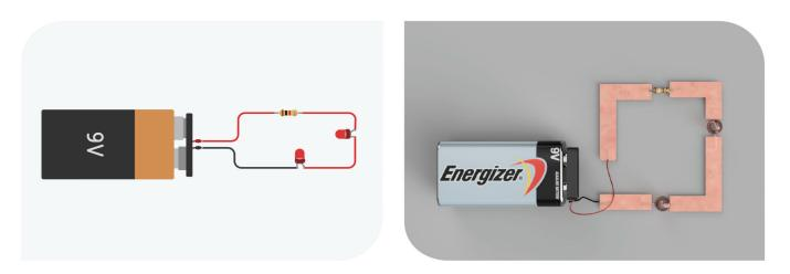
• Each component is connected in a line (ie. end to end). If the path is interrupted at any point, the whole circuit fails. Eg. water heaters, lamps
