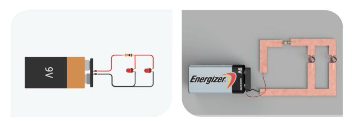
• Each component has its own path to ground. If one path is interrupted, the intergity of other path is not compromised. Eg. household wiring
