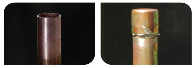
• Using the other piece of 4.5" copper pipe attempt to solder without applying flux. Note the behaviour of the solder
