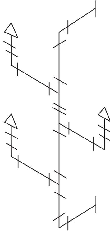
**Figure 23**—Isometric drawing of piping and bottle lamp. An open-headed arrow is used to represent a light bulb.
