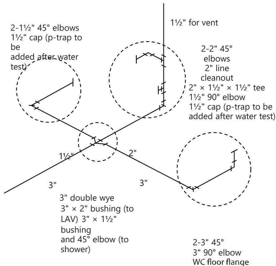
**Figure 24**—Rough in isometric
