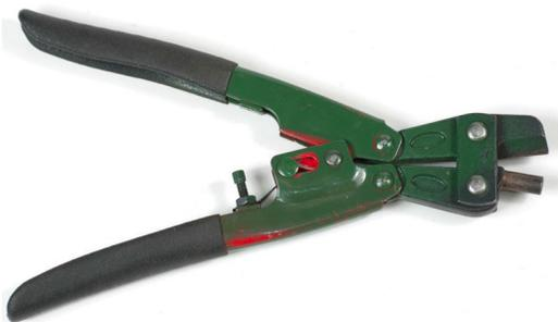
**Figure 3**—Crimp ring cutter
