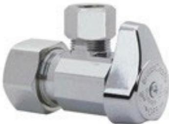
**Figure 6**—A compression-style CR 19 will fit over copper pipe. The chrome nut is then tightened to compress a brass ring, providing a watertight seal.
