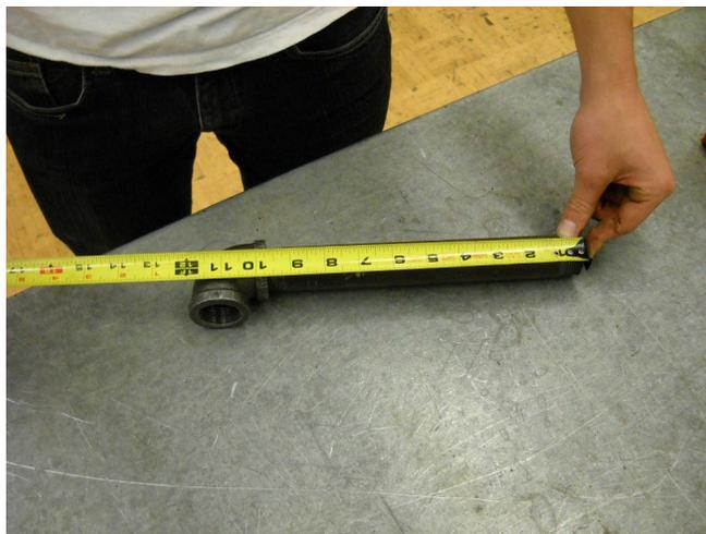
**Figure 7**—Care should be taken to keep the hook of the tape measure on the end of the pipe.
