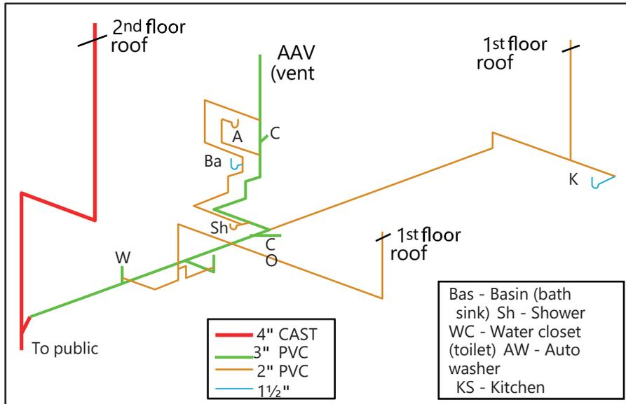
**Figure 17**—Isometric drawings allow a tradesperson to accurately determine how systems will be integrated and what supplies will be necessary for construction.
