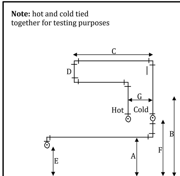
**Figure 19**—Crimping rough-in: front view
