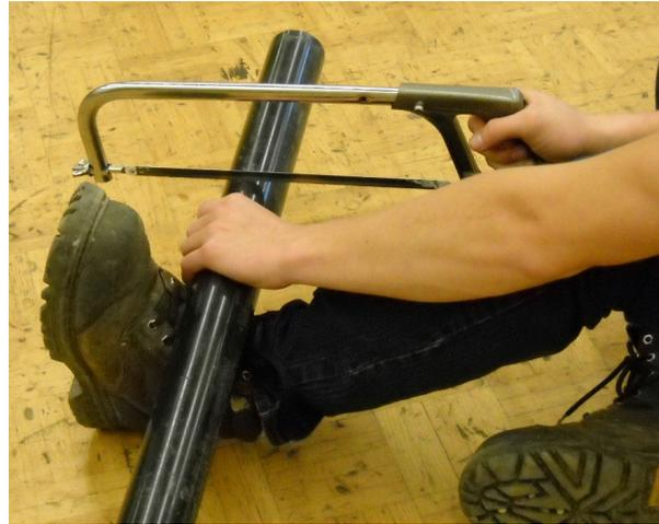
**Figure 14**—Cutting ABS in a seated position
