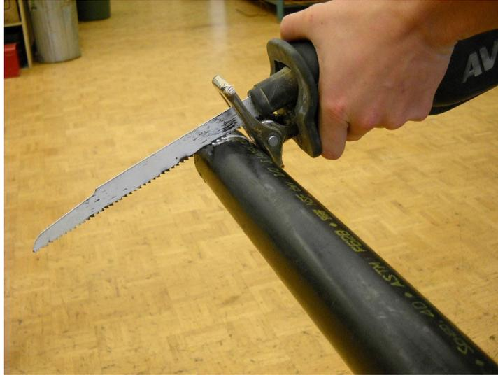
**Figure 18**—Reciprocating saws cut ABS pipe very quickly.
