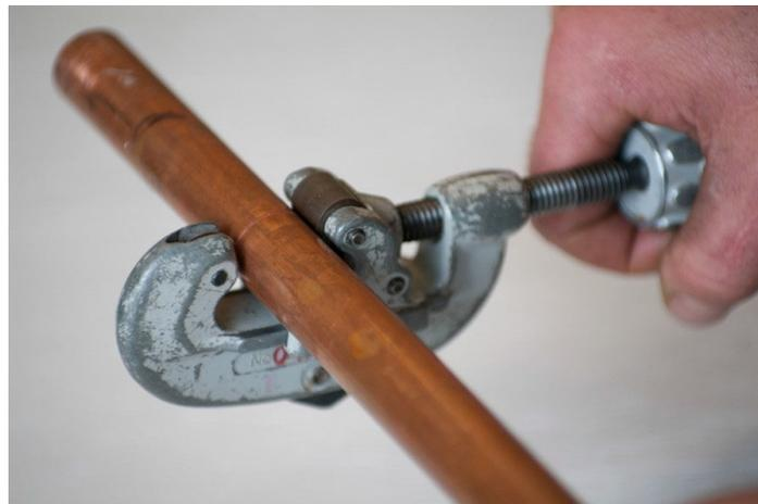
**Figure 1**—Tubing cutters ensure a straight, square cut.
