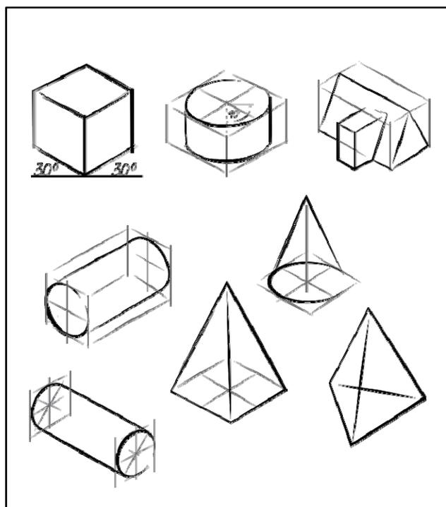
**Figure 19**—More complex shapes can be created by creating wire frames or boxes to which detail is added.
