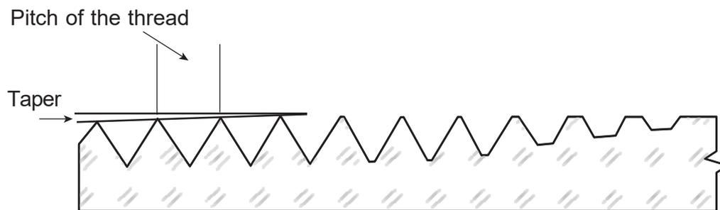
Figure 10—Close-up of tapered pipe threads
