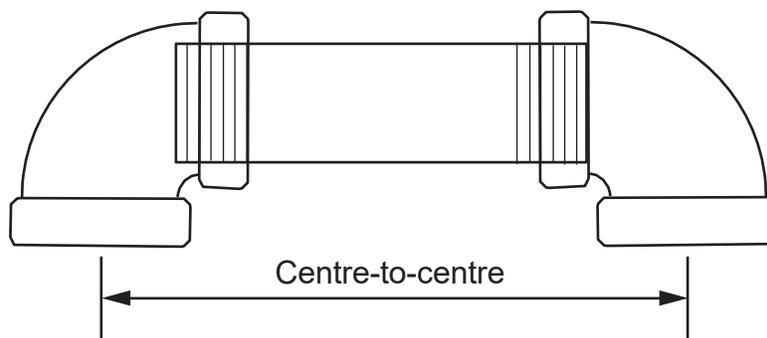
**Figure 5**—In most cases, centre-to-centre dimensions are used in plumbing
