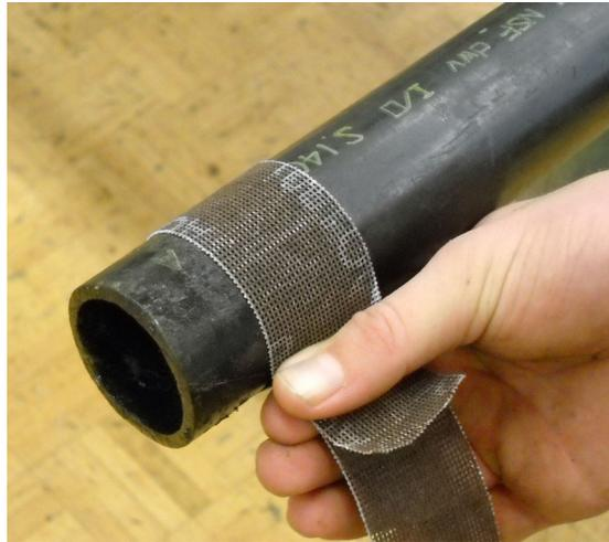
**Figure 16**—Positioning a wraparound to mark the cut line.
