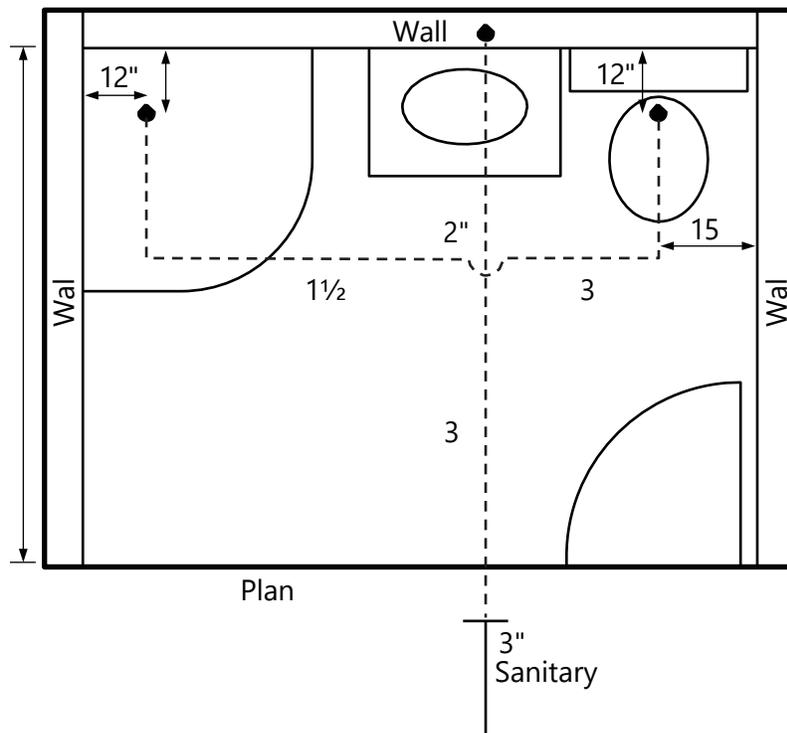
Figure 23—ABS rough-in (key)
