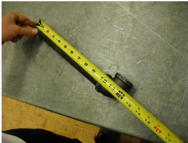
**Figure 6**—Correctly taking an end-to-centre measurement.
