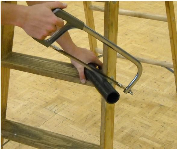
**Figure 13**—Cutting ABS with only a ladder support can be challenging at first.
