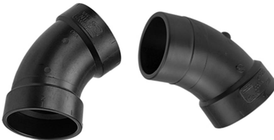
**Figure 3**—ABS 45°. The hub by hub 45 shown on the left connects two pieces of piping. The hub by spigot 45 shown on the right fits directly into another fitting (typically a wye).
