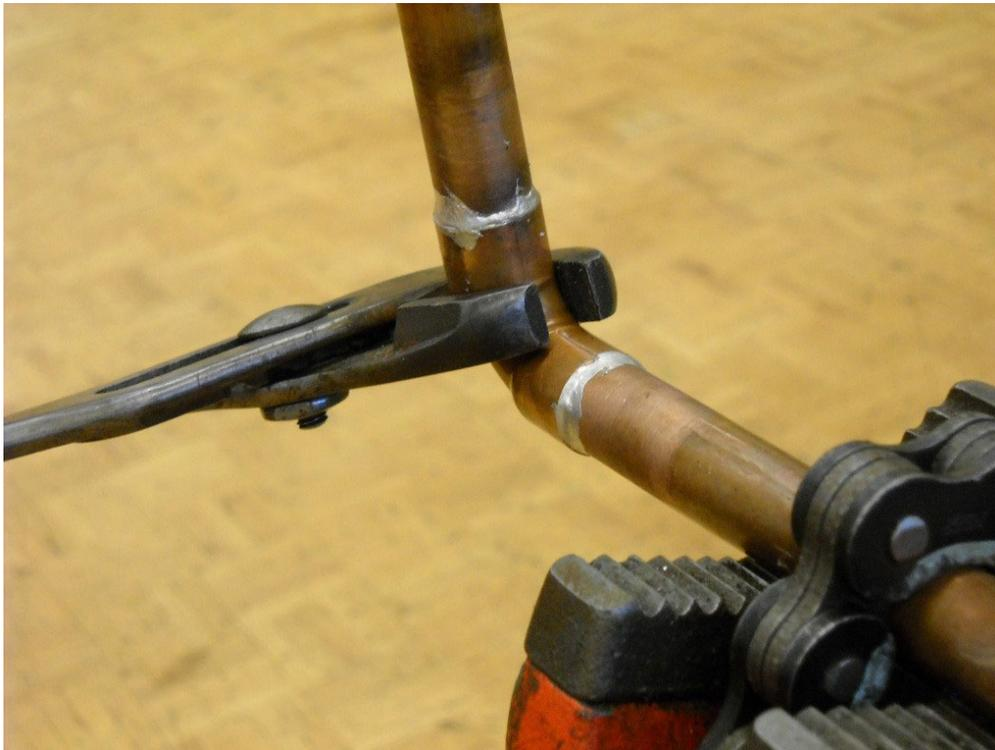
**Figure 8**—Copper fittings should be grasped at the corner so they don't bind on the pipe.
