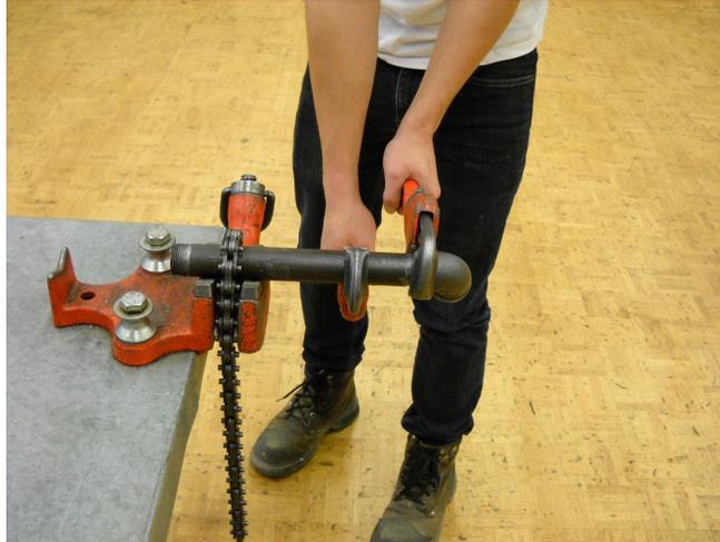
**Figure 9**—The chain vise is only used to support the work. The tightening of the fitting is accomplished by moving the two wrenches in opposite directions.
