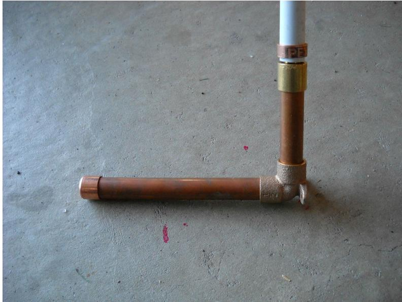
**Figure 12**—An adapter can be used to connect the copper outlet pipe to a PEX piping system.
