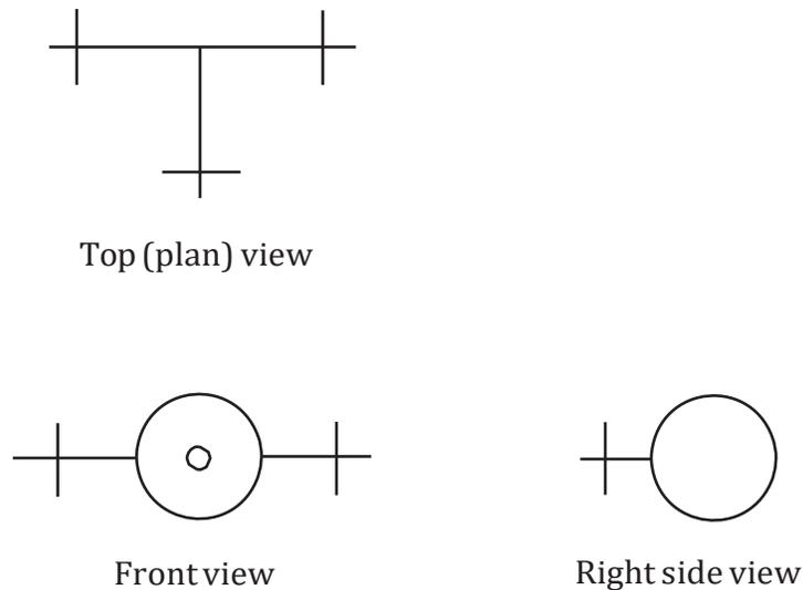
**Figure 10**—Orthographic projections for tee fitting in Figure 9
