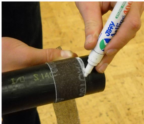
**Figure 17**—Marking a square line helps novices to produce square cuts.
