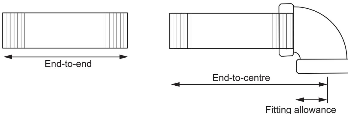
**Figure 4**—End-to-end, end-to-centre, and fitting allowance
