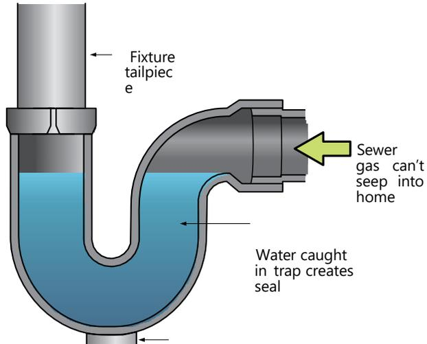
**Figure 10**—A cutaway view of a p-trap. Note that p-traps may have a cleanout plug to allow for cleaning or inspection of the piping. A solid p-trap is used if the trap is located in location that is not easily accessible (for example, a crawlspace).
