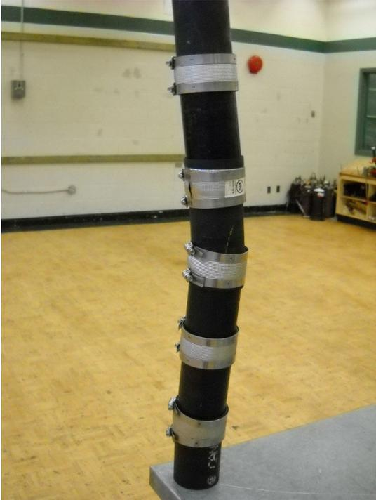
**Figure 9**—Poor practices generate a tower that is unstable.
