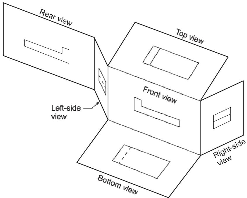
**Figure 5**—Views in an orthographic drawing
