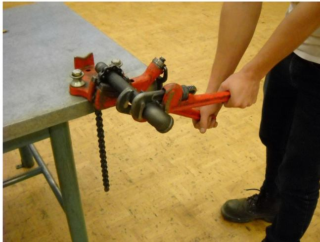
**Figure 8**—Controlled movement of pipe wrenches is accomplished with two wrenches and good hand placement.
