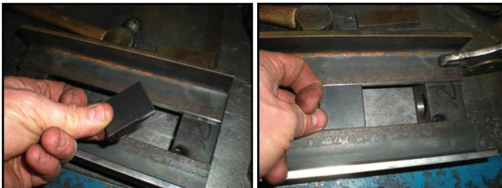
21. Grind spacer V-groove, position sliding jaw using spindle and nut, then tack weld spacer in position.
