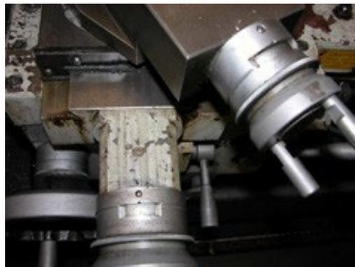
h. Make cuts engaging threading dial only at No. 1 position for a 13 TPI cut or according to the lathe manufacturer's instructions.
