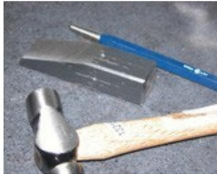
Centre-punch handle hole and retainer pin hole 6.5 mm offset from handle hole.
