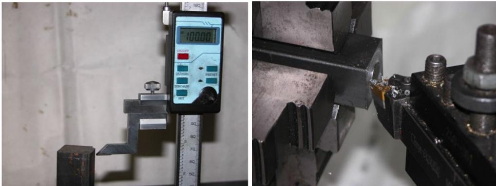
Then face the opposite end to approximate final length using lathe.
