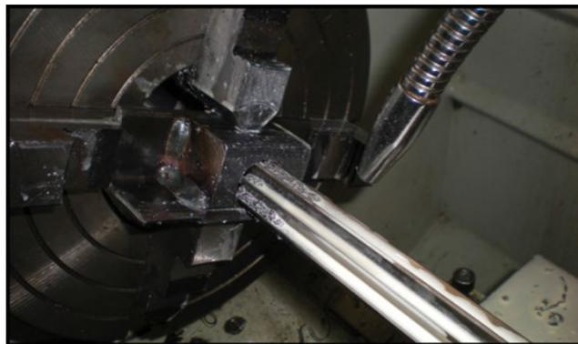
18. Spindle nut holder completed
