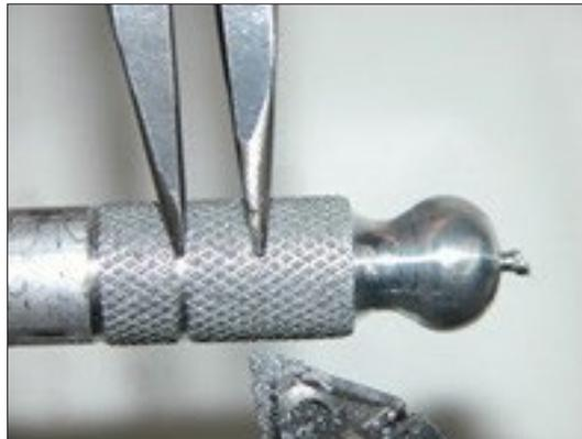
7. File (use lathe file), then sand (320 g) non-knurled section of body.
