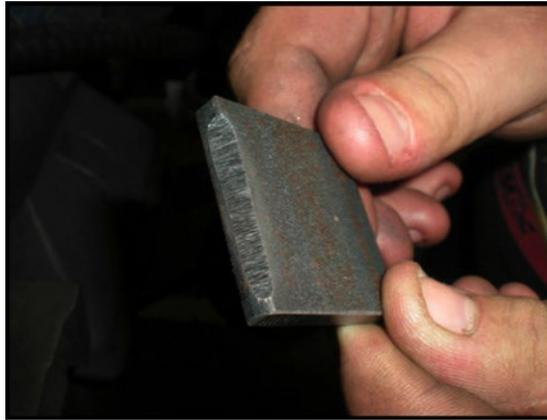
22. Remove sliding jaw from frame. Fill weld the V-groove and grind weld flush with edges.
