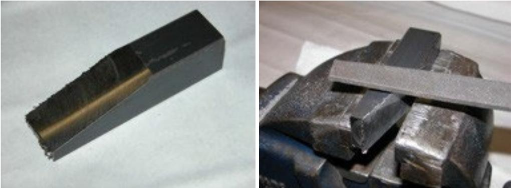
7. Side mill cross peen end to 30 degrees (option: grind and file to 30 degrees). Use a  $\frac{3}{4}$ " or larger 4-flute end mill. Hold down hammerhead to bed using a clamp kit as shown.
