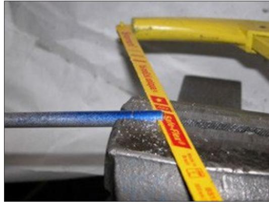
2. File smooth and flat. Cut off to length. File thicker end smooth with sharp edge and then slightly chamfer end.
