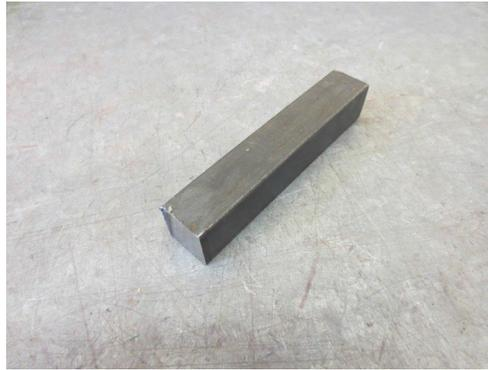
15. File all flat surfaces of the bar stock for the legs. This will make sure there are good contacts for welding at the assembly stage. Set the pieces aside.
