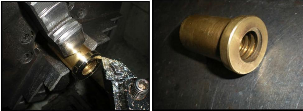
Completed bronze nut with chamfered edges
