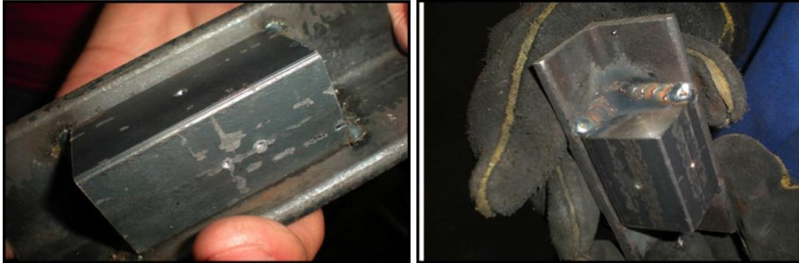
13. Drilling the sliding jaw:
