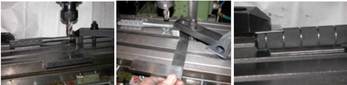
13. Touch the end mill to the top of the nut boss, then zero the knee height adjusting dial. Lock the x axis of the mill bed, provide clearance between the end mill and the nut boss, and raise the knee by 1.6 mm.
