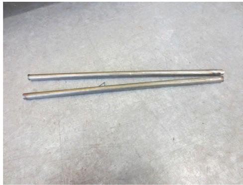
19. Measure and lay out two lengths of  $\frac{3}{16}$ " bar stock  $5\frac{3}{4}$ " in length. These pieces will eventually be welded to the grill for reinforcement.
