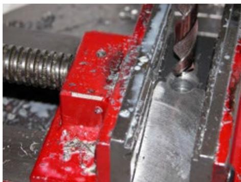
14. Using a 12-13NC tap, thread 27/64" hole through the head. Check to ensure that the tap is square to the hole throughout the process. Use appropriate tapping fluid.
