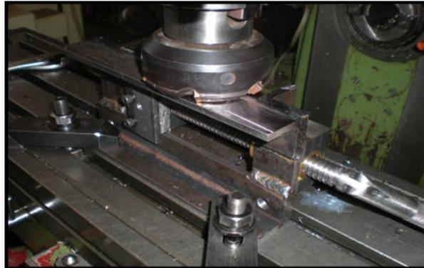
33. . Mill the ends or grind and file flat.
