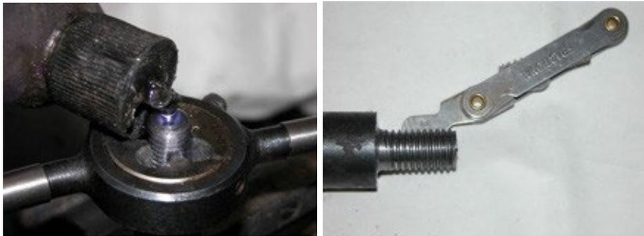
7. Turn a shoulder to  $0.600" \pm 0.005"$  × 3 mm wide at end of thread so that the hammer handle threads into the counter bore.
