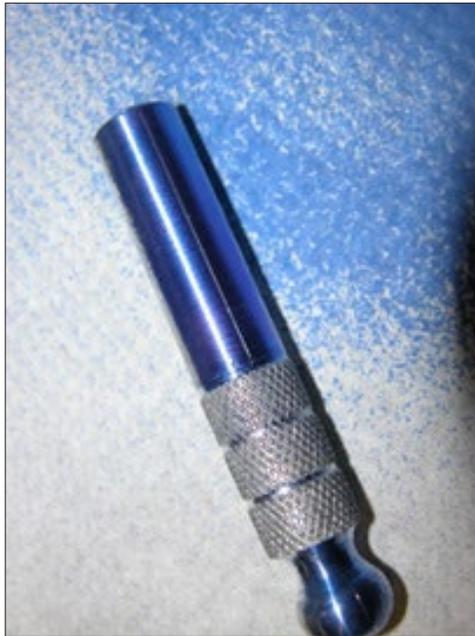
Mark off heights 18 mm from flat end and 6–7 mm from ball end.
