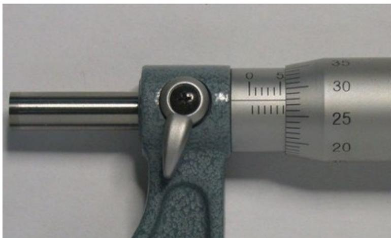
Metric micrometer's sleeve and thimble
