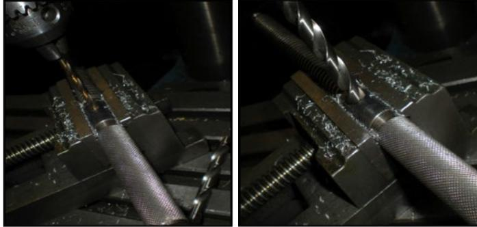
13. Round off ends of spindle and handle to semi-circular. Test fit with a  $\frac{3}{16}$ "  $\times$   $\frac{3}{4}$ " round head rivet so that 90-degree motion right and left is possible.
