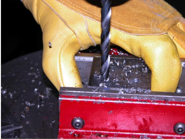
**Figure 9**—Drill at each centre-punched point
