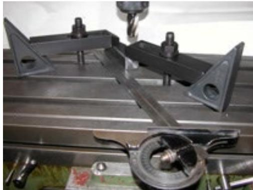
8. Zero cross y axis dial when material touches overhanging end of hammerhead. Cut 2 mm off of end at a 30-degree angle. Flip the head over and repeat on the other side.
