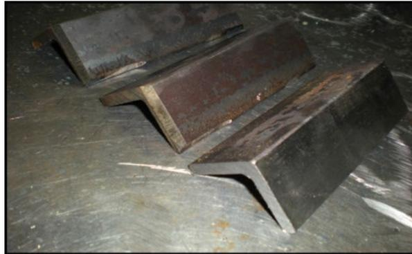
3. V-groove ends of side rails for welding; belt on top surface only.
