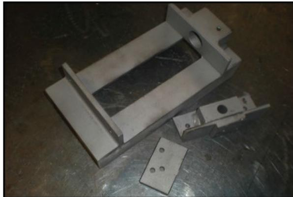
3. Mask off contact areas on the sliding jaw and rails.
