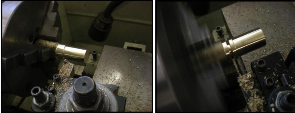
2. Reverse nut in lathe chuck, centre drill, pilot drill at  $\frac{1}{4}$ ", bore through at  $\frac{39}{64}$ ".
