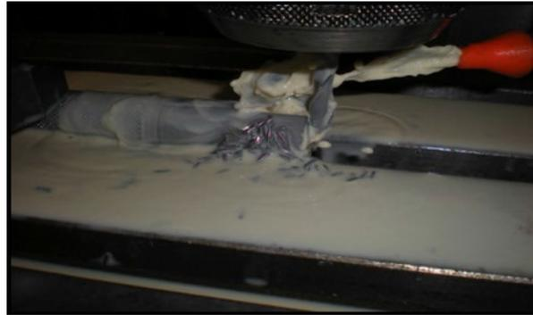
Make successive  $\frac{1}{8}$ " passes until end mill is through the diameter of the handle.
