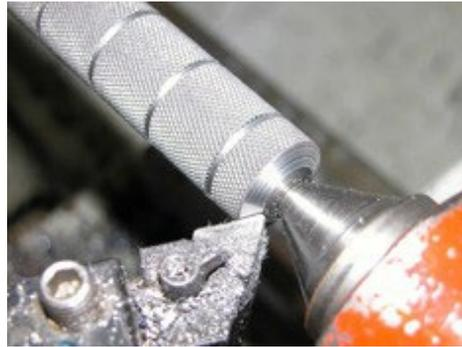
11. Chamfer each side of the nut boss. Support part using tailstock and live centre.
