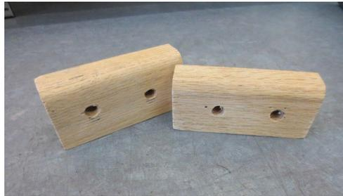
**Note:** Countersink procedure has not been completed in this image.
