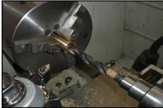
3. Set lathe feed to 6 TPI, remove tool post, set rpm to about 50, align tandem Acme  $\frac{3}{4}$ -6 tap with live centre in tailstock, turn 3 revolutions by hand, keeping tap in contact with live centre while running through. Posi-drive with tap bar or wrench.
