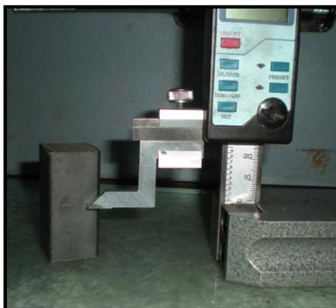
8. Grind off one edge of both blocks to allow blocks to sit tightly against the angle iron. Chamfer ends of blocks using a flat file.
