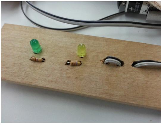
**Figure 8**—Wood LED mount - front
