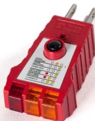
**Figure 3**—Plug (receptacle) tester
