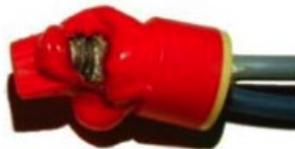
**Figure 5—**Result of a high-resistance fault.
