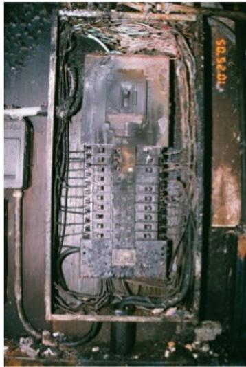
**Figure 9**—Result of overload in an electrical panel
