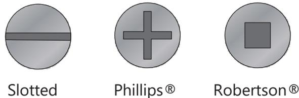
**Figure 7**—Types of screwdrivers
