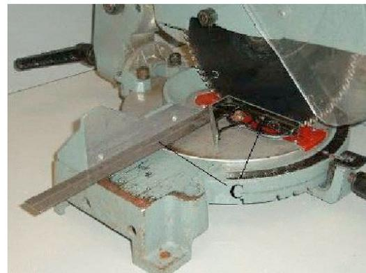
**Figure 24**—Fence adjustment 2
