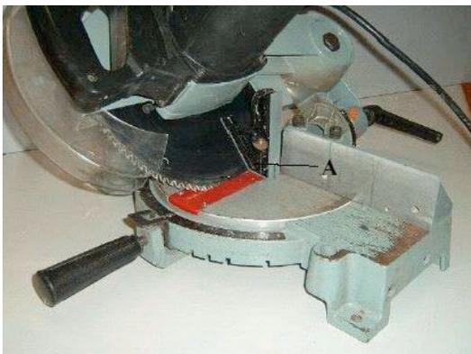
Figure 20—Bevel adjustment 3
