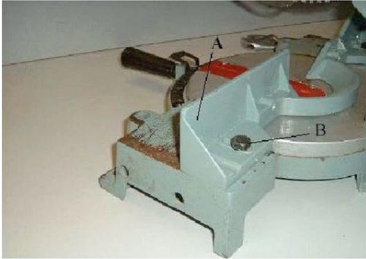
**Figure 14**—Fence in forward position
