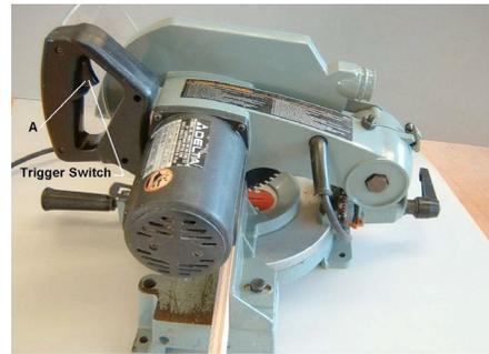
Figure 9—ON–OFF trigger switch
