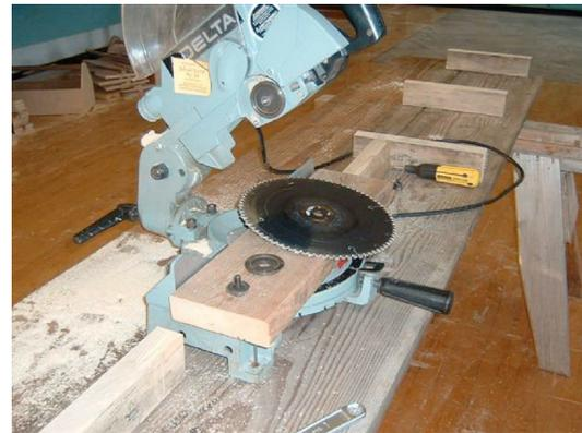
Figure 33—Blade removal
