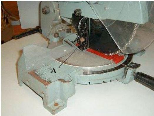
Figure 18—Bevel adjustment 1
