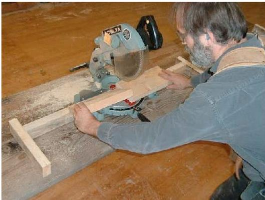
**Figure 16**—Checking bevel error
