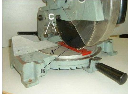
**Figure 22**—Blade parallel to blade insert opening in tabletop
