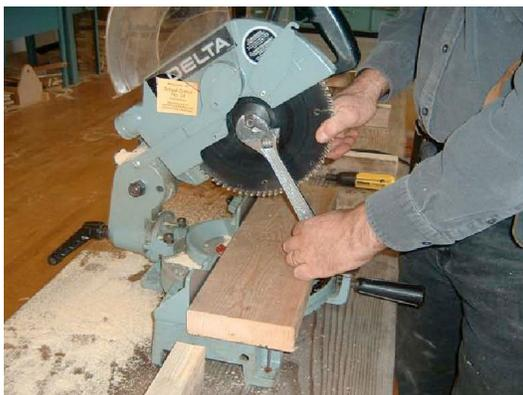
Figure 34—Blade installation
