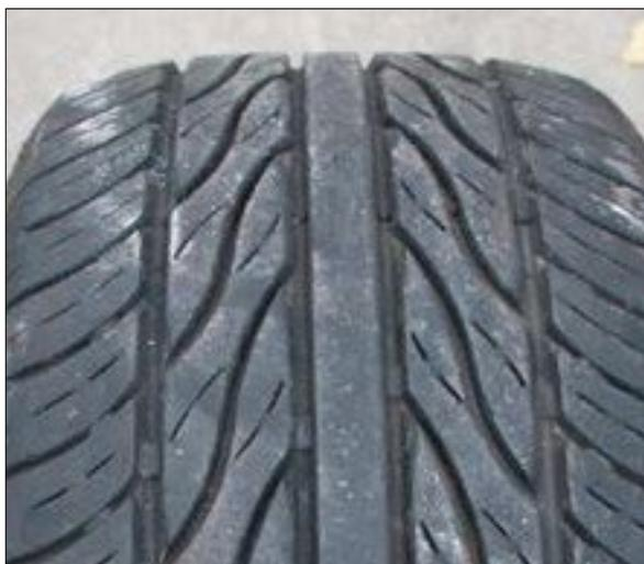
**Figure 4**—Siped directional tire
