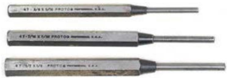
Figure 12—Drift punches
