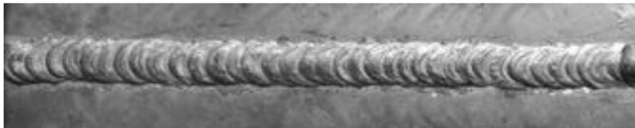
**Figure 8**—Weld bead formed correctly
