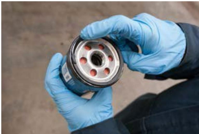
**Figure 6**—Lubricate the new oil filter seal
