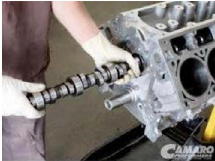
**Figure 16**—In-the-block camshaft
