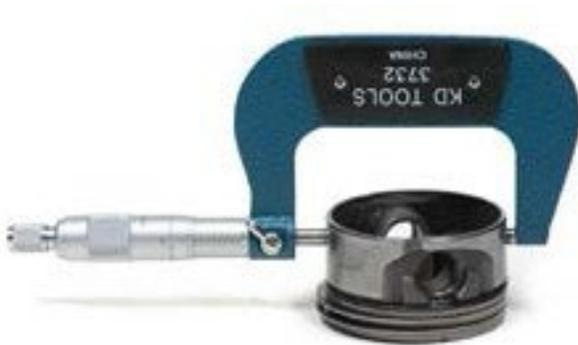
Figure 2—Measuring a piston
