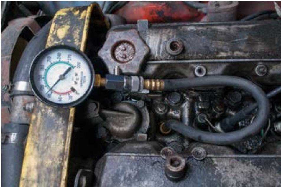
**Figure 9**—Compression gauge inserted into spark plug hole
