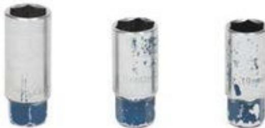
**Figure 40**—Spark plug socket wrench
