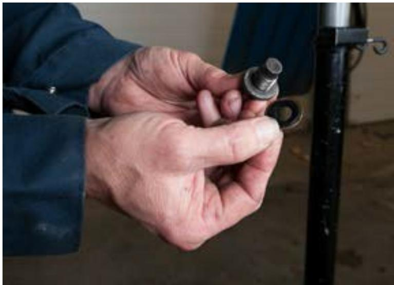
**Figure 2—Drain plug seal**
