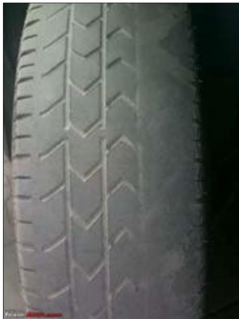
**Figure 19**—Tire wear from toe-in or toe-out
