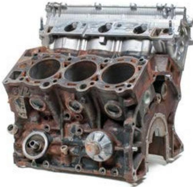
**Figure 1**—Cylinder block with head attached
