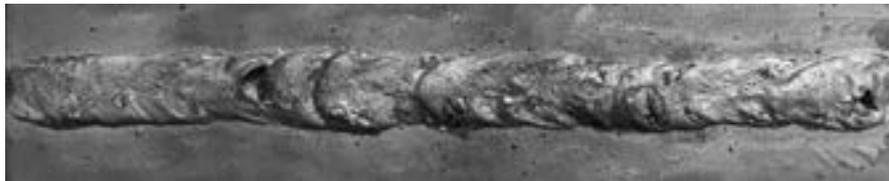
**Figure 7**—Weld bead formed with too much heat
