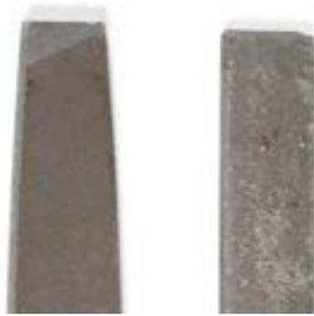
**Figure 16**—Files with tapered and blunt end
