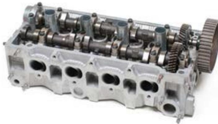
**Figure 17**—Camshaft located over the head
