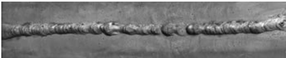
**Figure 5**—Weld bead formed when speed of travel was too fast
