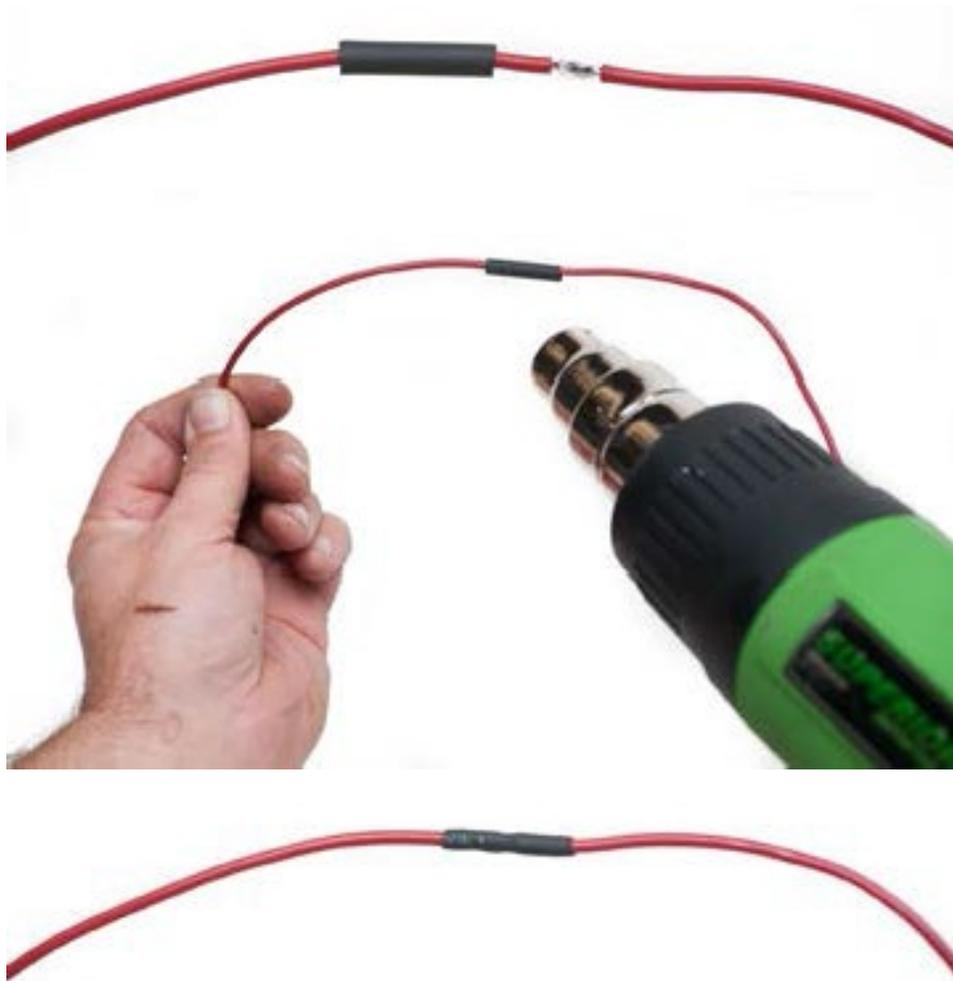
**Figure 7**—Applying heat shrink to a soldered joint
