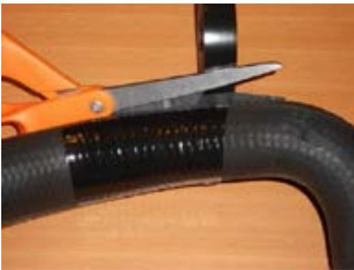
**Figure 11**—Cutting the electrical tape
