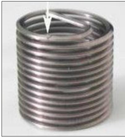
**Figure 6**—Inverted HeliCoil insert
