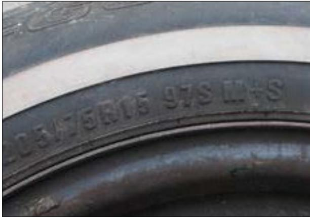
**Figure 1**—Mud and snow (P) passenger tire
