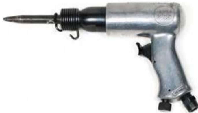
**Figure 8—Air chisel**
