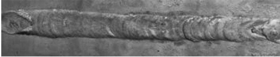
**Figure 6**—Weld bead formed when speed of travel was too slow
