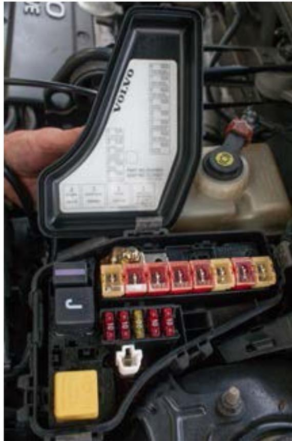
**Figure 6**—Typical fuel pump relay location
