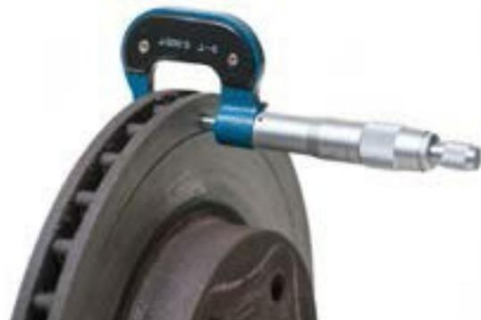
Figure 3—Measuring a brake rotor
