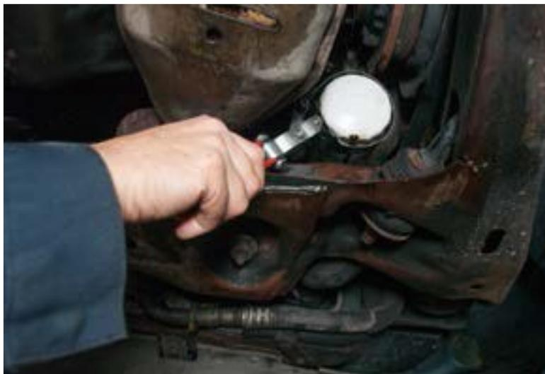
**Figure 4**—Remove oil filter
